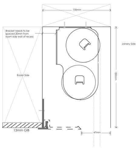
VANDA PART BOX EXTRUSION WITH EXTENSION COVER PLATE **PART No. VA-FB-105**
